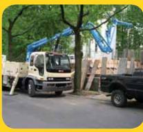
incorporates welding seams below the edge of maximum stress. The boom is engineered to offer the flexibility to adapt to different loads and features more straight pipe for a less stressful concrete flow and longer wear on parts. The Z-Fold configuration handles space restrictive areas and can pump even if the boom is not fully extended.
