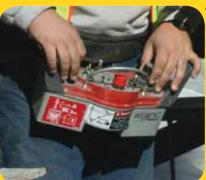
ensures minimal interference with other frequency transmitters. Radiomatic Power Boost further enhances recention quality with a 50-100% increase in signal power. A fully proportional cable remote is also standard. Unlike other remote control systems, the radio and cable remote systems are completely independent, offering redundancies to ensure complete proportional operation
