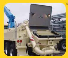
Putzmeister's EZ Clean Out RS 905A hopper is engineered for performance and easy maintenance. Offering 19.4 cu. ft. (550L) capacity, the hopper features hard-faced remixer paddles and vibrator. The splash guard design protects the unit from splattering during pumping and folds down and latches to cover the hopper during transit.
