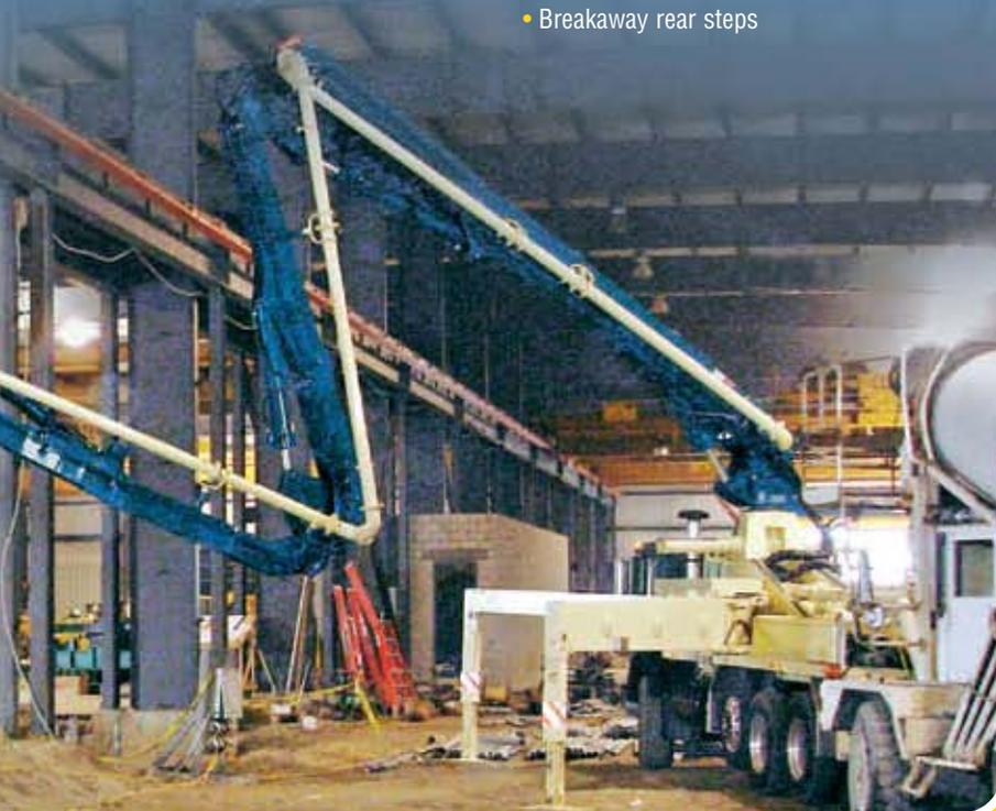
to maximize the reach of each boom section to obtain precise concrete placement. The model's low 18 ft. 9 in. unfolding height and boom flexibility enable the operator to maintain a single location throughout a job while preventing the need for extra delivery line.
